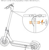
2. Firmly connect the wires inside the handle and the stem. Slide the handle onto the stem. Be aware of the correct orientation
