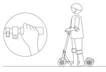
DO NOT press the throttle when walking with the KickScooter.
