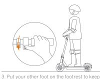
both feet stable. Press the throttle on the right hand to speed up when you are balanced.
