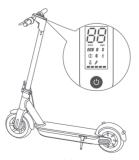
Power on the KickScooter and check the power level indicator. Charge the KickScooter if the battery level is low.
