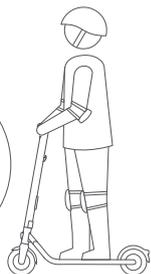
3. Put your other foot on the foot deck to keep both feet stable. Press the throttle on right hand to speed up when you are balanced.
