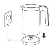
Close the lid. Position the kettle on the power base in place. Make sure the kettle contact with the power base completely. Then the indicator light will turn on to show the current water temperature.
