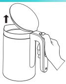
■ To fill water into the kettle, remove it from the power base and open the lid by press down the lid opening button, fill with the desired amount of water to the kettle. Always fill the kettle between the minimum (0.5L) and maximum (1.5L) marks. Too little water will result in the kettle switching off before the water has boiled.
