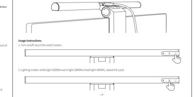
3. Turn the lamp body to adjust the lighting angle and complete the installation.
