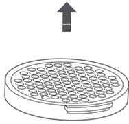
2. Place the filter on top of the cyclone assembly and gently push it into place, while pushing aside the safety clip on the left side of the notch.
