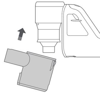
5. Gently push the dust compartment in the direction as shown in the figure until you hear a click, indicating that the compartment has been firmly secured.
