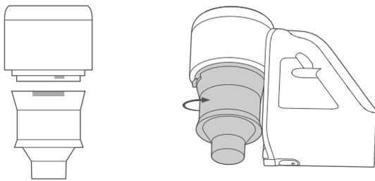
4. Slightly tilt the dust compartment when installing it on the vacuum.
