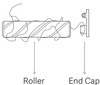
4. After cleaning, install the end cap back on the roller.
