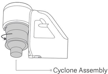
3. Remove the internal filter from cyclone assembly.
