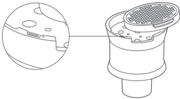
3. Align the cyclone assembly with the vacuum as shown in the figure, and turn the cyclone assembly in place by turning it clockwise.
