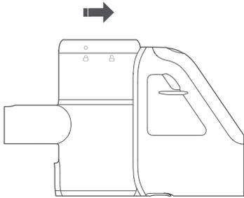
2. Rinse the inside of the top filter under the tap. Rotate the filter while rinsing it to make sure that all the dust in the filter gaps is rinsed out. Tap the filter several times against the sink to remove all the remaining dust before rinsing it.
