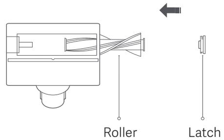
6. With the side latch of the brush head facing your direction, use a coin to turn the latch clockwise into the locked position, while making sure the roller is in place.
