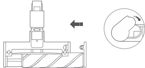
6. Rotate the latch clockwise by 90° to the locked position to secure the roller.
