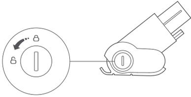
2. After removing the latch, remove the roller from the bed attachment.
