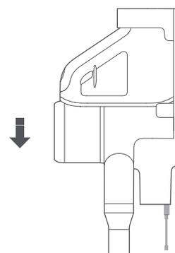
Pull the vacuum down in the docking station to charge
