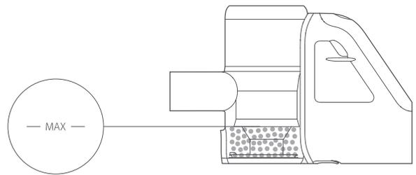
2. To empty the dust compartment, push the switch on the dust compartment in the direction of the arrow to open the bottom cover and empty it into a trash can.
