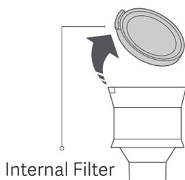
4. Rinse the filter and cyclone assembly until they are clean. Wring out the filter after rinsing.
