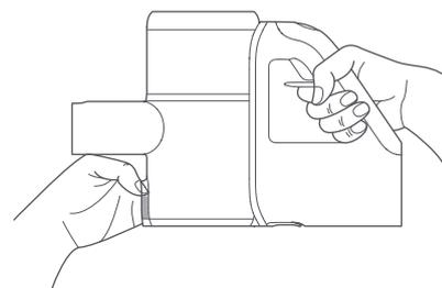
3. While pushing the switch next to the dust compartment in the direction of the arrow, pull the compartment away from the vacuum to rinse it with water.
