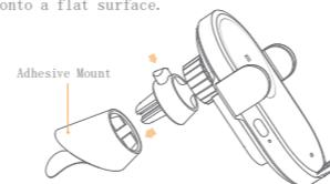
Note: The surface for mounting the wireless car charger needs to be clean and flat. Make sure to press and hold it firmly for 5 to 10 seconds after mounting. Due to the strength of the adhesive, forced removal may damage the car's interior. It is recommended to have a professional to remove the adhesive mount.
