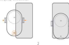
3. In order to achieve a better charging performance, make sure the phone is properly placed onto the wireless car charger, so it is close to the charging surface (refer to the figure below). When the indicator blinks, it indicates that the charger is in protection mode. Please check whether there is a metal object on the charging surface or on the back of the phone. If the issue persists, please contact after sales
