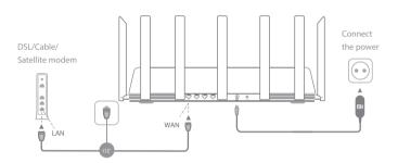
Power on the router, then connect the Internet (WAN) port to the DSL/Cable/satellite modem
