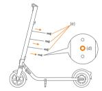
4. Install the external battery on the rail. Fixate the two M4 screws (with 3 mm hex wrench) and the M3 screw (with 2.5 mm hex wrench). Block the screw holes with the rubber stopper when installed.
