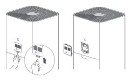
Note: To avoid damaging the purifier, do not rinse or spray the filter compartment directly with water, or wipe it with a soaking wet cloth.
