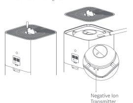
Note: To avoid damaging the purifier, do not rinse or spray the air duct and fan blades directly with water, or wipe them with a soaking wet cloth.
