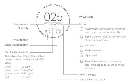
The negative ion function is enabled by default. The purifier can generate negative ions when it is working, and then the negative air ions (NAI) are produced through the reaction between the negative electron and the oxygen molecules. NAI is very good at trapping certain air pollutants. The function can be enabled or disabled in the app. When it is enabled, the negative ion indicator is on; when it is disabled, the indicator is off.
