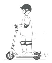
12.To change the center of gravity when turning, turn the handle slightly.
