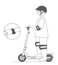
11.Release the acceleration handle to reduce speed, and squeeze the brake lever to brake.
