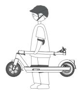
③Hold the fronttube to lift the electric scooter.
