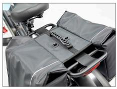
4. Put the bag on and lock the knob by 90 degrees.
