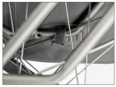
5. Fix the strap securely on the back of the bag to the rack.
