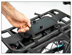
2. After adjusting the position, tie the straps around.
