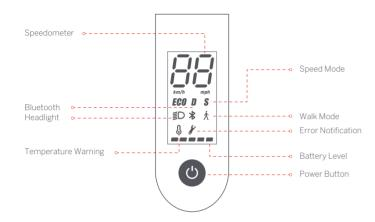
Power Button: Press the button to turn on; press and hold the button for 3 seconds to turn off. When the KickScooter is on, press the button to turn on/off the headlight and the rear light, and press twice to switch between the speed modes.
