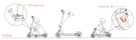
Release the safety hook, and push the quick-release lever down. Then fold the stem.
