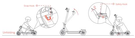
Disengage the snap hook from the buckle.
